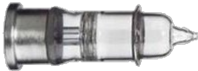
Fig. 1 DC discharge excitation lamp
